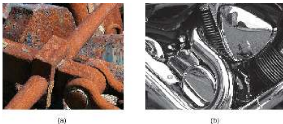
Figure 1.19 (a) One of the chemical properties of iron is that it rusts; (b) one of the chemical properties of chromium is that it does not. (credit a: modification of work by Tony Hisgett; credit b: modification of work by "Atoma"/Wikimedia Commons)
