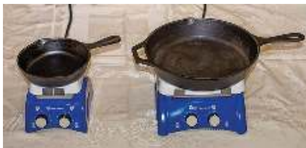
Figure 5.8 Because of its larger mass, a large frying pan has a larger heat capacity than a small frying pan. Because they are made of the same material, both frying pans have the same specific heat. (credit: Mark Blaser)
