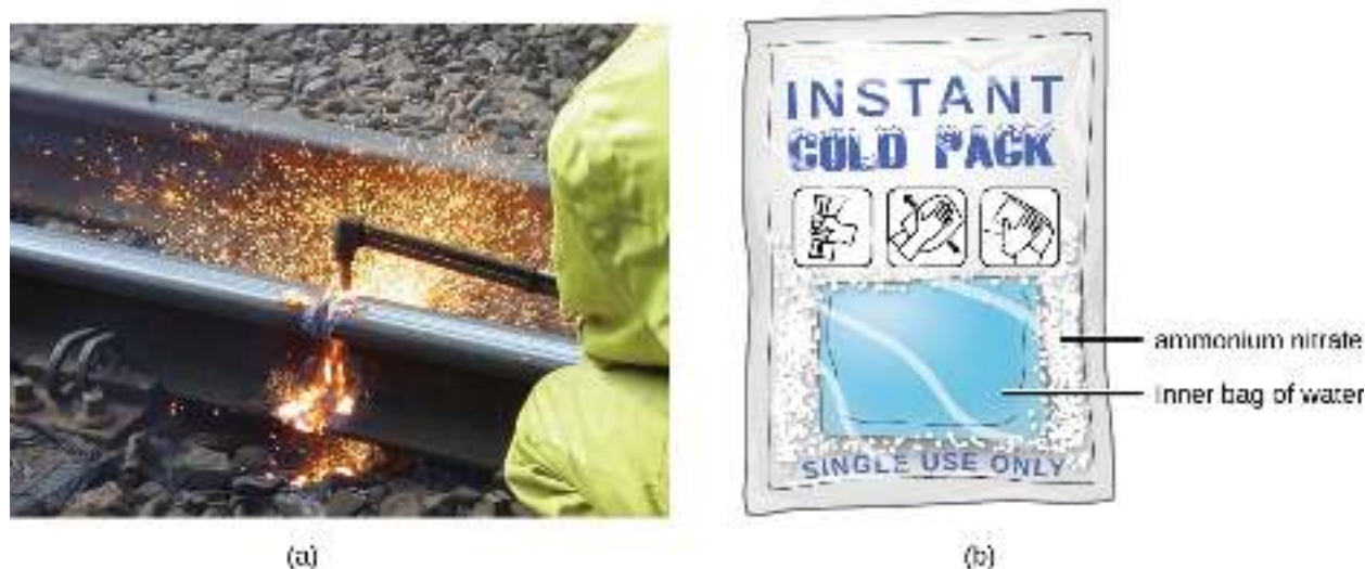
Figure 5.7 (a) An oxyacetylene torch produces heat by the combustion of acetylene in oxygen. The energy released by this exothermic reaction heats and then melts the metal being cut. The sparks are tiny bits of the molten metal flying away. (b) A cold pack uses an endothermic process to create the sensation of cold. (credit a: modification of work by “Skatebiker”/Wikimedia commons)
