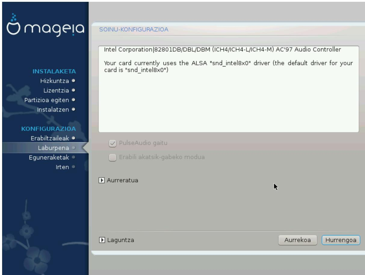
This screen shows the details of the sound card driver chosen for you by the installer, and this driver should work without problems.
