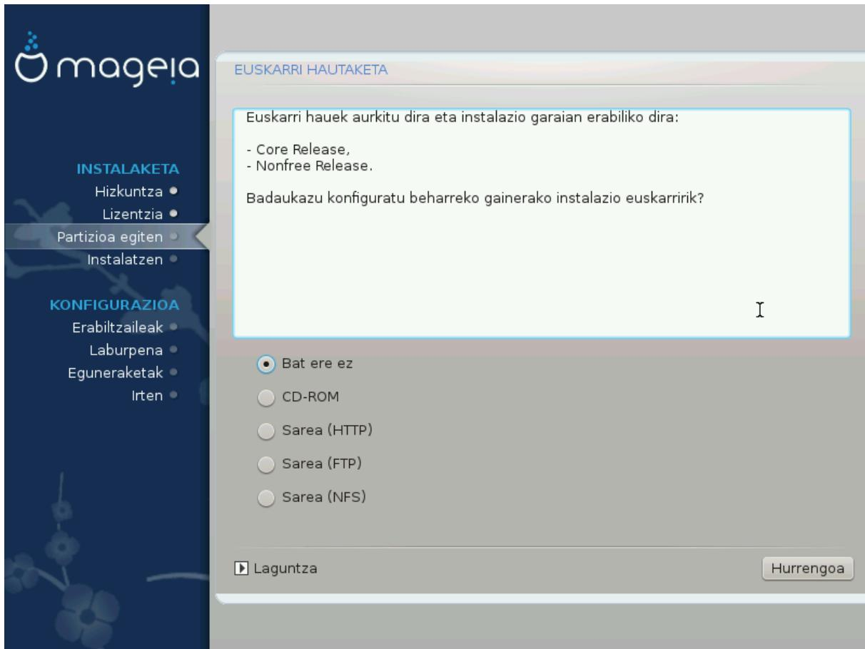
This screen shows you the list of already recognised repositories. You can add other sources for packages, like an optical-disc or a remote source. The source selection determines which packages will be available during the subsequent steps.
